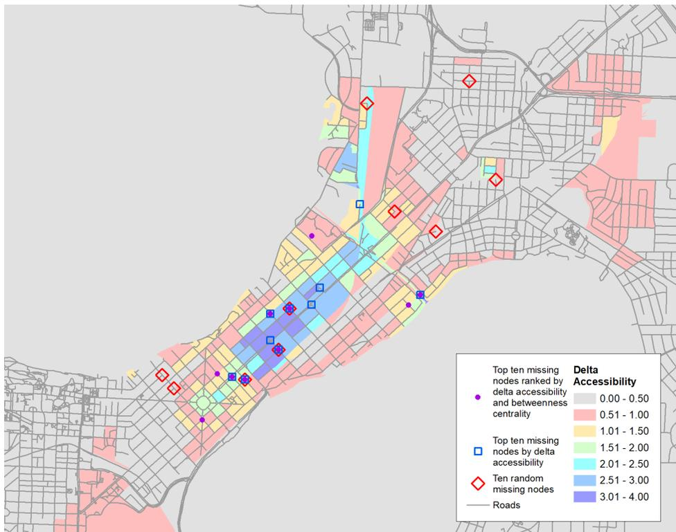
Figure 4. Missing ramp intersections selected by three methodologies.
