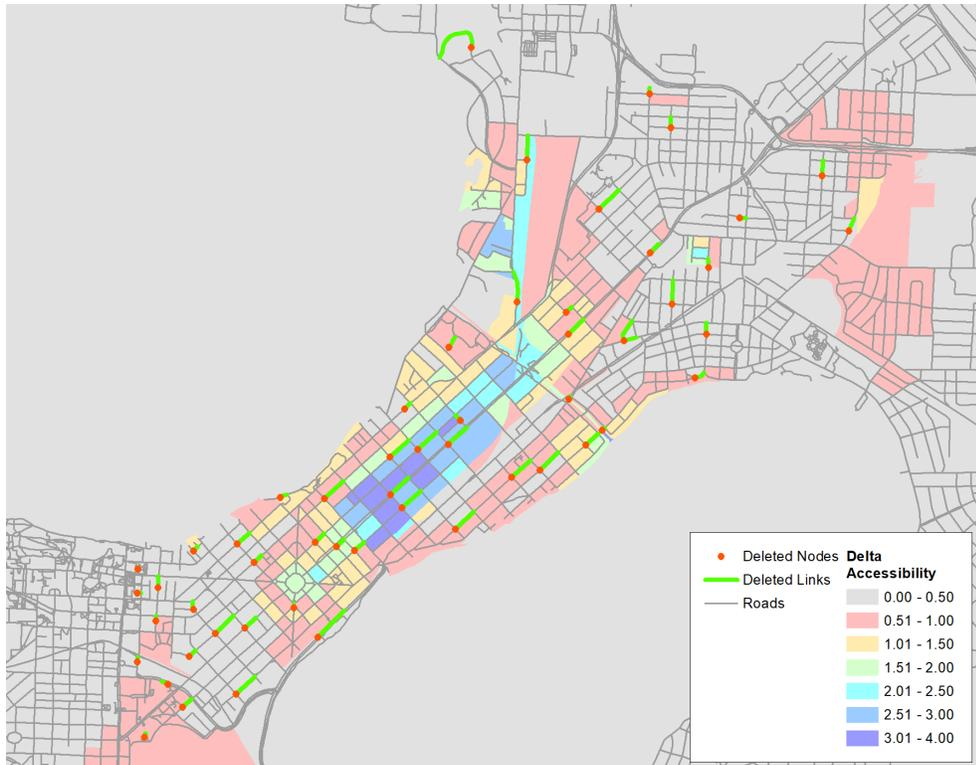
Figure 1. Links removed from continuous network to approximate missing ramps.
